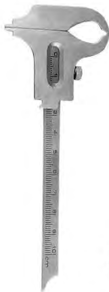
Fig.2 TM-126-1873 Boley Measuring range 0-100 mm
